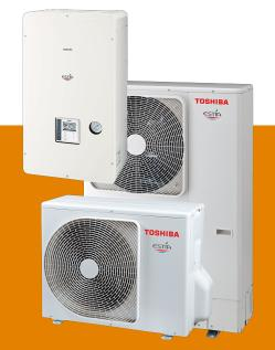
Air/Water heat pumps in a split design for flow temperatures up to +55°C, in the power range of 5 to 16 kW, for generating hot or cold water. Combination of outdoor unit and hydro unit for supplying all applications such as hot water tanks, fan coils, radiators, or underfloor heating.
